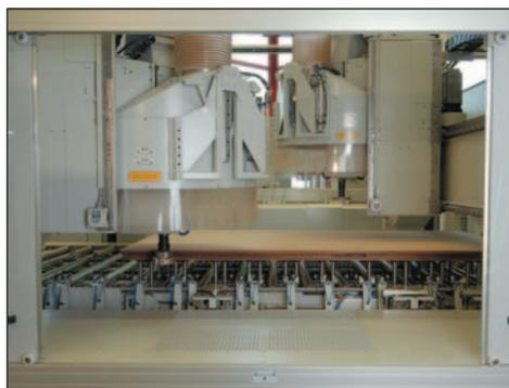
*Two independent 5-axis heads machine on a through-flow pin table with individual sinkable vacuum pins.*
