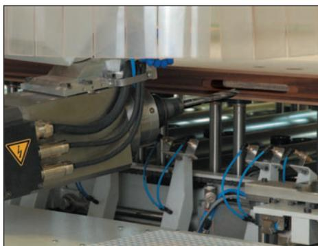
*Both five-axis heads are capable of working at up to 8 degrees below horizontal.*
