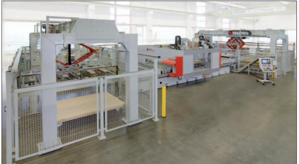
*Vision-UT Sprint door production cell with twin automatic loading portals and through-flow table will be demonstrated on the Reichenbacher Hamuel stand at Ligna 2009.*
