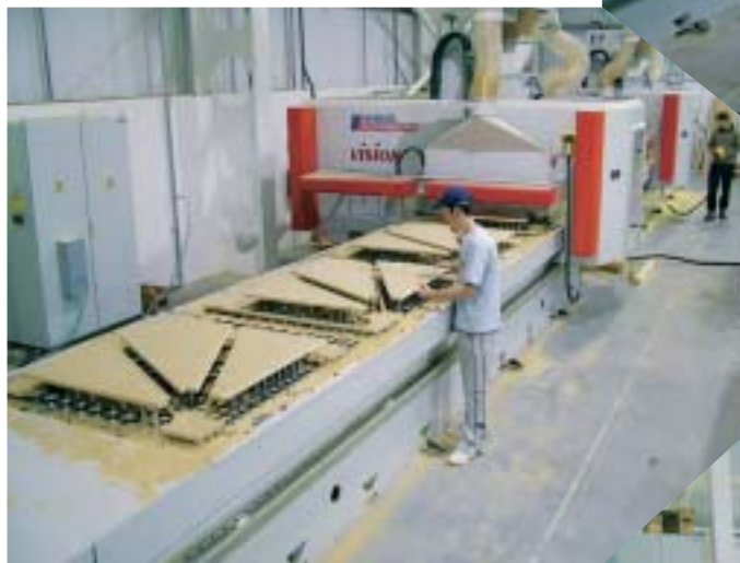
Twelve winder plates produced in just 12 minutes, including set-up, on the Hamuel Reichenbacher custom-built Vision Sprint
