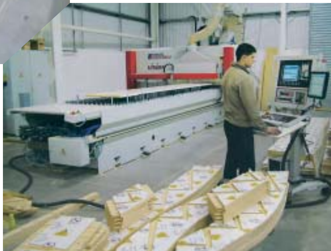
Pin-table configuration reduces set-up time for machining strings to just seconds.
